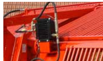
Option: Oil cooler to cool oil in transmission case
