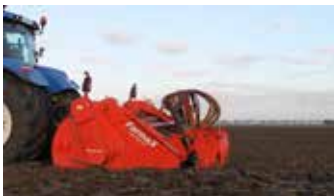
Tilling depth up to 16.69" (50 cm)
